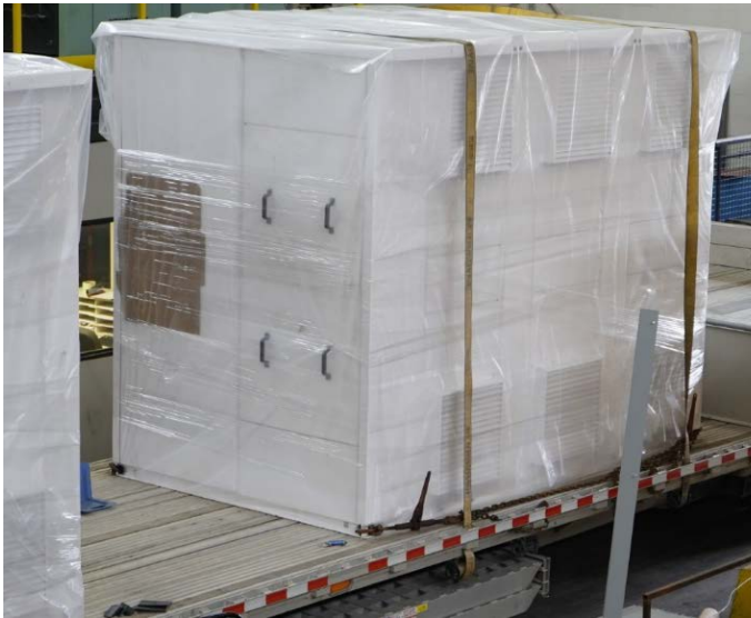
Figure 1: Typical Enclosed Transformer Shipment Packaging (Shown with Tarp Removed)
