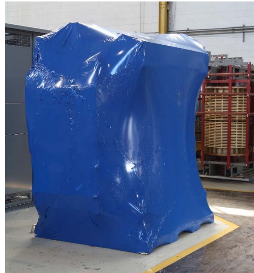
Figure 2: Typical Core & Coil Transformer Shipment Packaging with Shrink Wrapping
